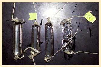
• This worked great. Not only did the dialysis tubing expand when oxygen was generated, but it also changed color showing the secondary reaction.
