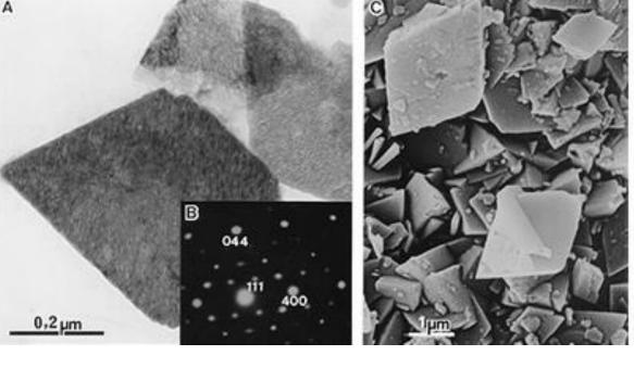
SEM of alpha alumina  $(AI_2O_3)$  [1]
