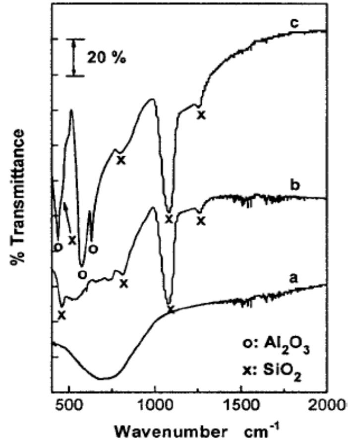
FIG. 1. FTIR spectra of prepared aluminum oxide films on Si substrates: (a) recorded from as-deposited films by ECR-PLD from a metallic Al target with oxygen plasma assistance, (b) recorded from films annealed at 1000 °C in air and (c) recorded from films annealed at 1100 °C in air.
