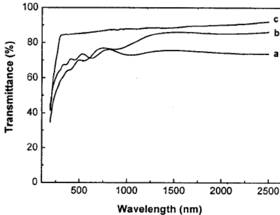
FIG. 4. UV and IR optical transmission spectra of (a) as-deposited aluminum oxide films on sapphire substrates and (b)  $\alpha$ -Al<sub>2</sub>O<sub>3</sub> films on sapphire substrates prepared by ECR-PLD and followed by heat annealing at 1100 °C in air. (c) For comparison, a transmission spectrum of a bare sapphire substrate is also displayed.
